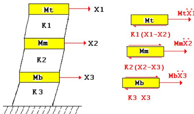
Figure 3: The 3DOF model (left) and the free body diagrams.
