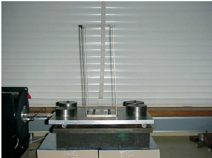
Figure 6: Deflection of the 1DOF structure.
