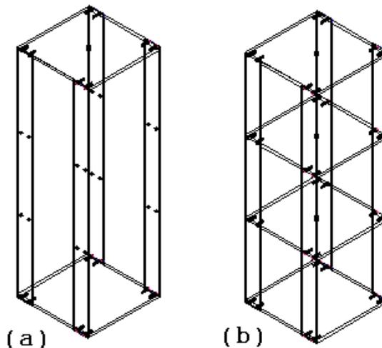
Figure 2: Wire Frame Models of the Structure, (a) 1DOF and (b) 3DOF.
