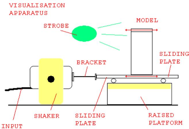
Figure 4: Visualisation experiment set-up.
