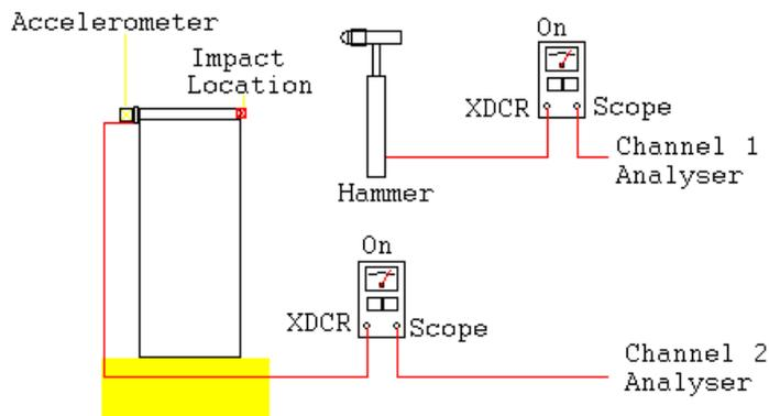
Figure 1: Measurement of a 1DOF structure's natural frequencies.
